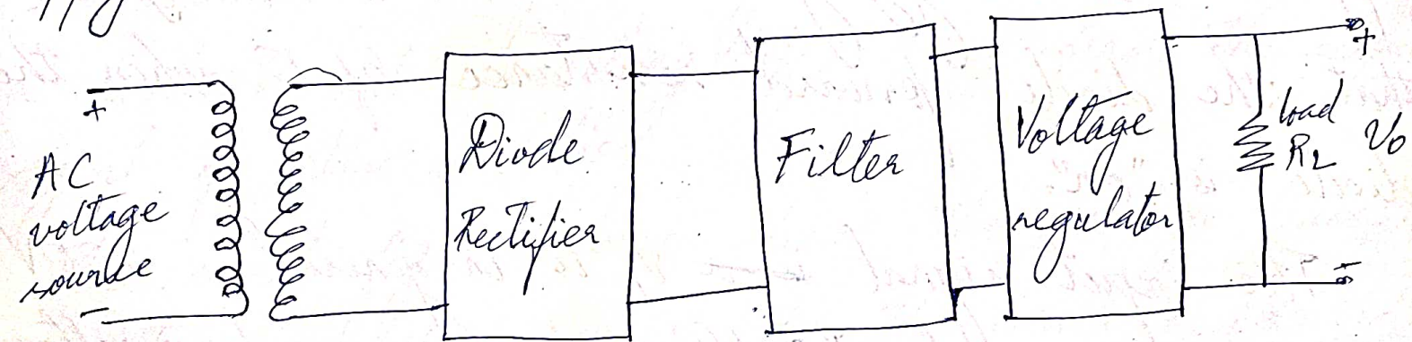
Diagram of an electronic power supply
